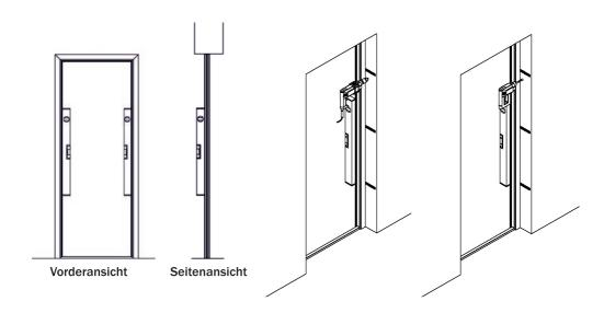
After the screwing check the level by air level. Fill up the space between the jamb and opening with mounting foam.
