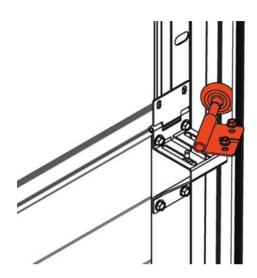
Insert a roller with 20mm spacer ring and a steel rope into the bottom corner brackets.
